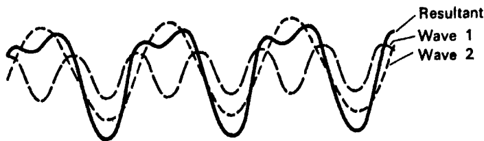
Figure 2-14. Complex wave formed by the algebraic addition of two different pure waves.
